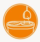
SPÜLBOY® glass washer combines spatially separated pre-washing and fresh water rinse systems in one device. This enables the application within one sink. At that SPÜLBOY® convinces with lowest and most efficient water consumption of 10cl per glass. A one-time initially filling is sufficient due to the continuous supply of fresh water released by each rinsing step.
